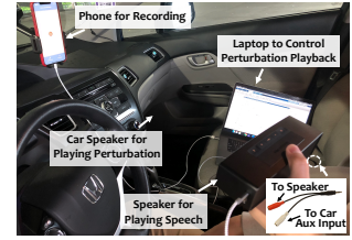
Figure 8: Illustration of the inside-vehicle setup.
